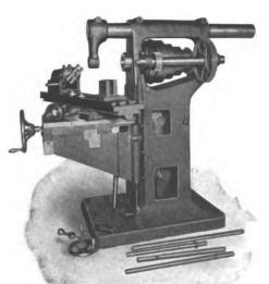
Figure 10. No. 3 Universal Milling Machine, with 20inch table travel and 17-inch vertical travel, now under construction.
