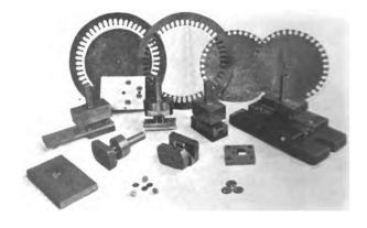
Figure 12. Photograph of a few punches and dies made by students
